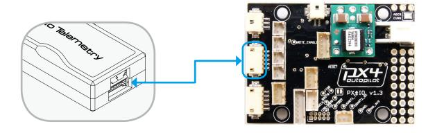
Connect to the PX4 I/O telemetry port using the 6-to-5-pin cable.
