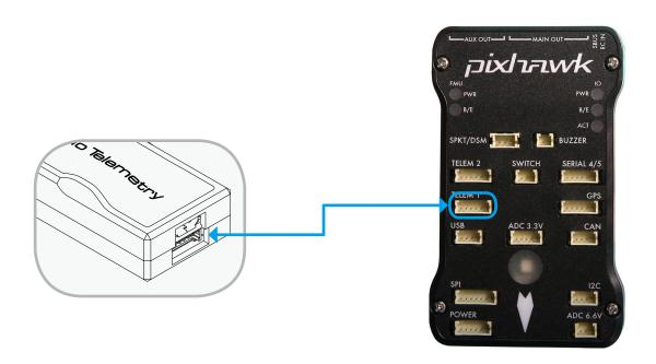
Connect to the Pixhawk telemetry port using the 6-pin cable.
