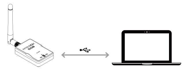
Use Micro-USB cable to connect ground module and a laptop loaded with ground station. You need to download the latest version of RTB BOX drive on the XROCK official website.
