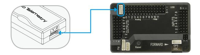
A Connect to the APM telemetry port using the 6-to-5-pin cable.
