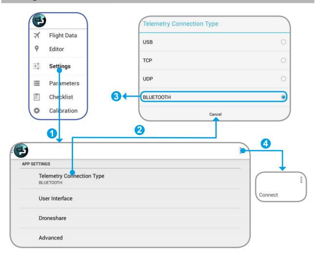
After Bluetooth pairing and air module installation is successful, operating DroidPlanner according to the picture. Select Connect, and air-to-ground data link can be realized.
